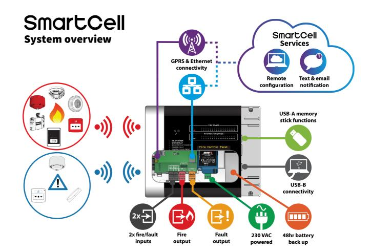
SmartCell has been designed as a complete wireless fire detection system to protect people and property. The system incorporates separate information zones which allow input devices to be configured in multiple configurations, providing maximum flexibility to the user and designer. In the event of an alarm, the system detects the alarm condition, raises the alarm, and also indicates the location of the fire via zone text and indication along with an individual device text description.
